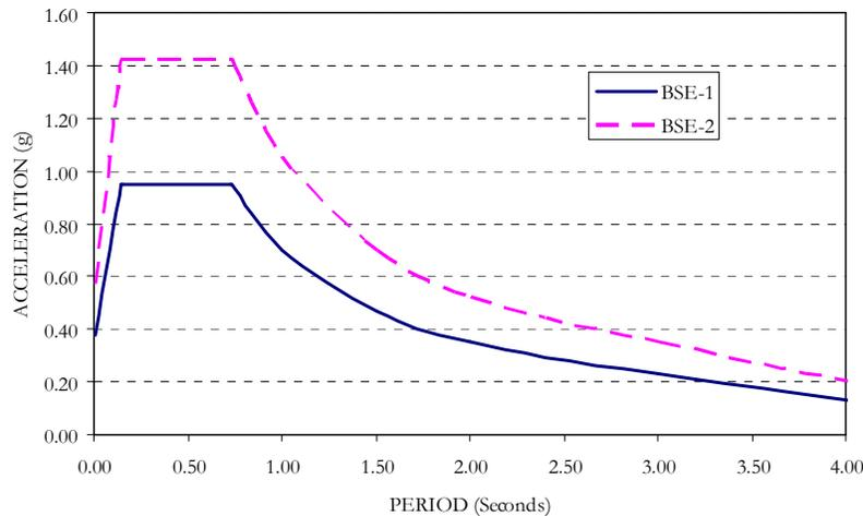
Figure 2: BSE-1 and BSE-2 5% Damped Design Spectra
