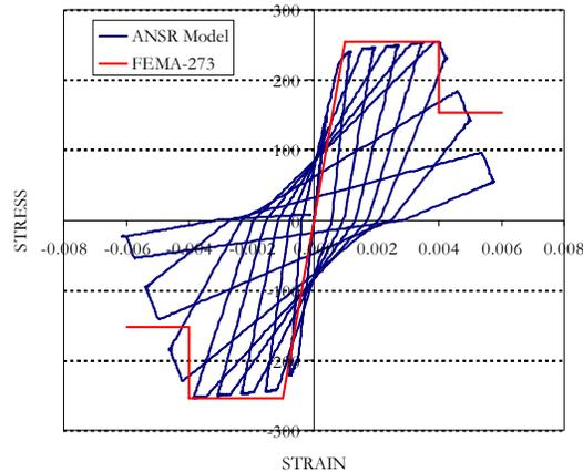
**Figure 2: URM shear hysteresis compared to FEMA recommendations**
